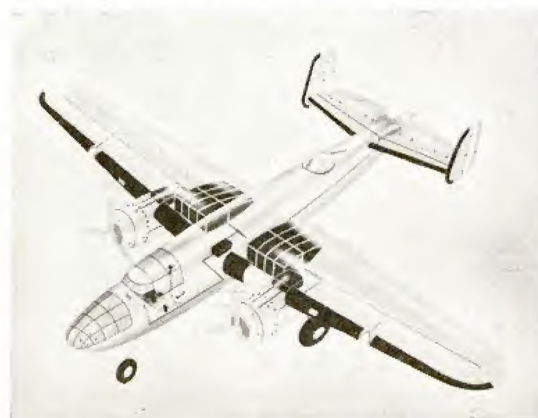
Black shading in drawing of American medium bomber marks parts of the ship where rubber must be used in its construction and its accessories
